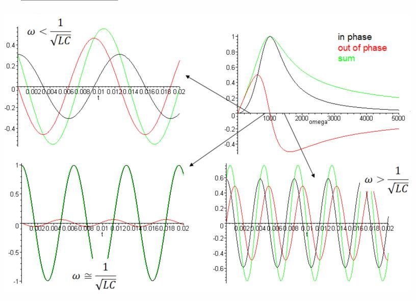
At any instant:  $v_d(t) = v_R + v_c + v_c = V_d \cos(w_d t)$ but  $v_R$ ,  $v_c$ , and  $v_c$  have different phases and must be added carefully.
