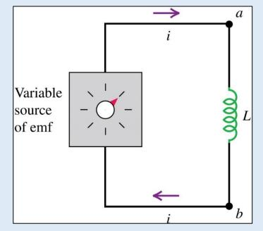
• Electric potential is defined in terms of conservative electric fields; follows that potential difference between inductor leads is
