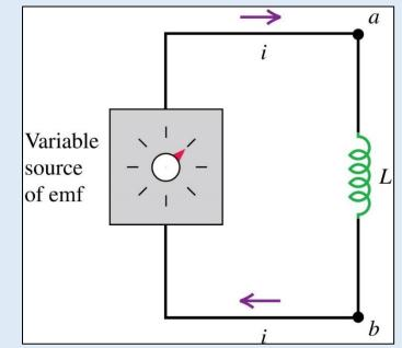
• Because  $\vec{E}_{nc} \neq 0$  is only between a and b, integrating the line integral in Faraday's law clockwise around the loop gives
