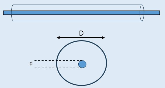
• The inner wire diameter d is 0.80 mm. The diameter D of the inside surface of the outer conductor is 5.0 mm. The insulator is non-magnetic.
